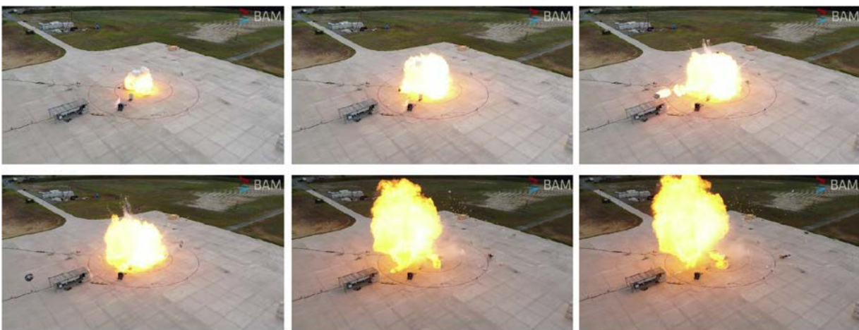
Figure 14: Test with horizontal vessel insulated with MLI: Fireball development.
