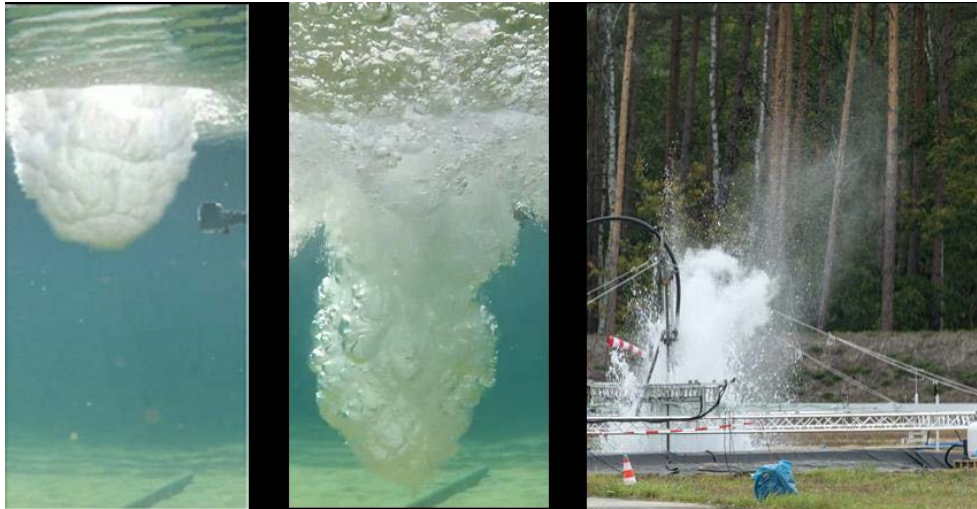
Figure 5: LH 2 jet penetrating the water (release rate 0.8 kg/s, release location 50 cm above the water surface pointing downwards). The left picture shows a moment shortly after the jet entered the water surface. The picture in the middle shows the penetration depth of the jet. The picture to the right shows the geyser-like behaviour over the water surface caused by the evaporating liquid hydrogen.
