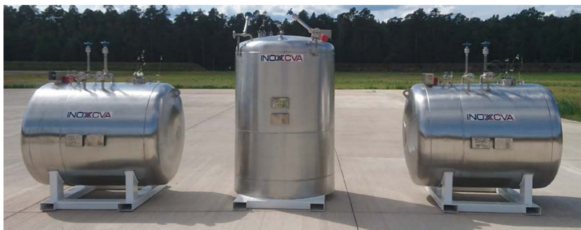
Figure 10: The three LH 2 storage vessels used during the BLEVE experiments.
