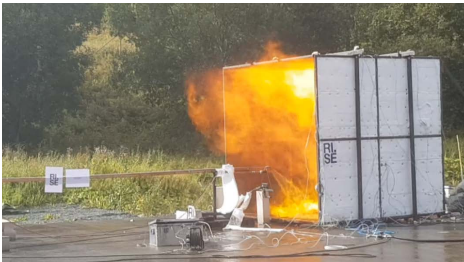
Figure 20: Enclosure configuration with 5 panels. Box with an open front face. The test shown is T16 (J45-5P) with the jet angled 45° down onto the floor panel approximately 1 second after ignition.
