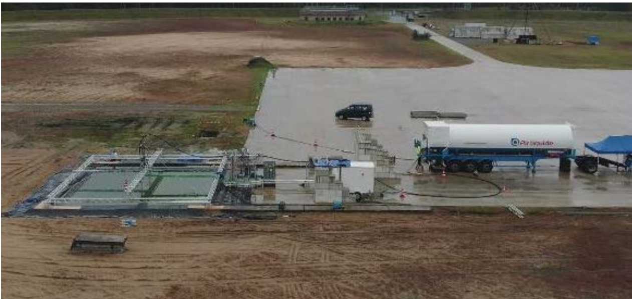
Figure 3: View of the test set-up to study the release of LH2 onto and under water. The picture shows the basin on the left with a bridge structure for holding the release mechanism and instrumentation. On the right the road trailer carrying the LH2. In the middle the cabin used for logging equipment.
