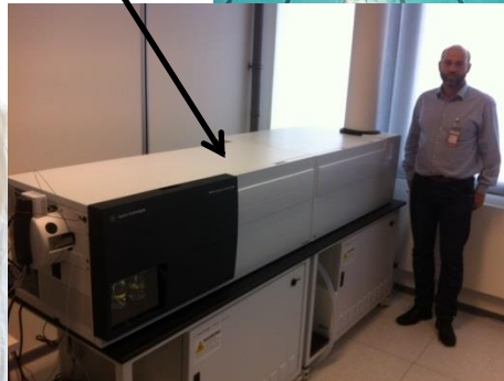
FT-ICR-MS ultra high resolution MS-identification. (Only instrument in Scandinavia, ca. 20 WW, of this class)
