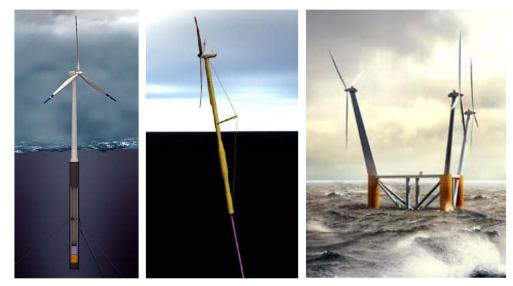
Figure 2 Floating concepts, from left: HyWind, SWAY and WindSea.
