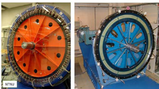
Figure 10 Lab-scale PM generators at NTNU (left) and SmartMotor (right).
