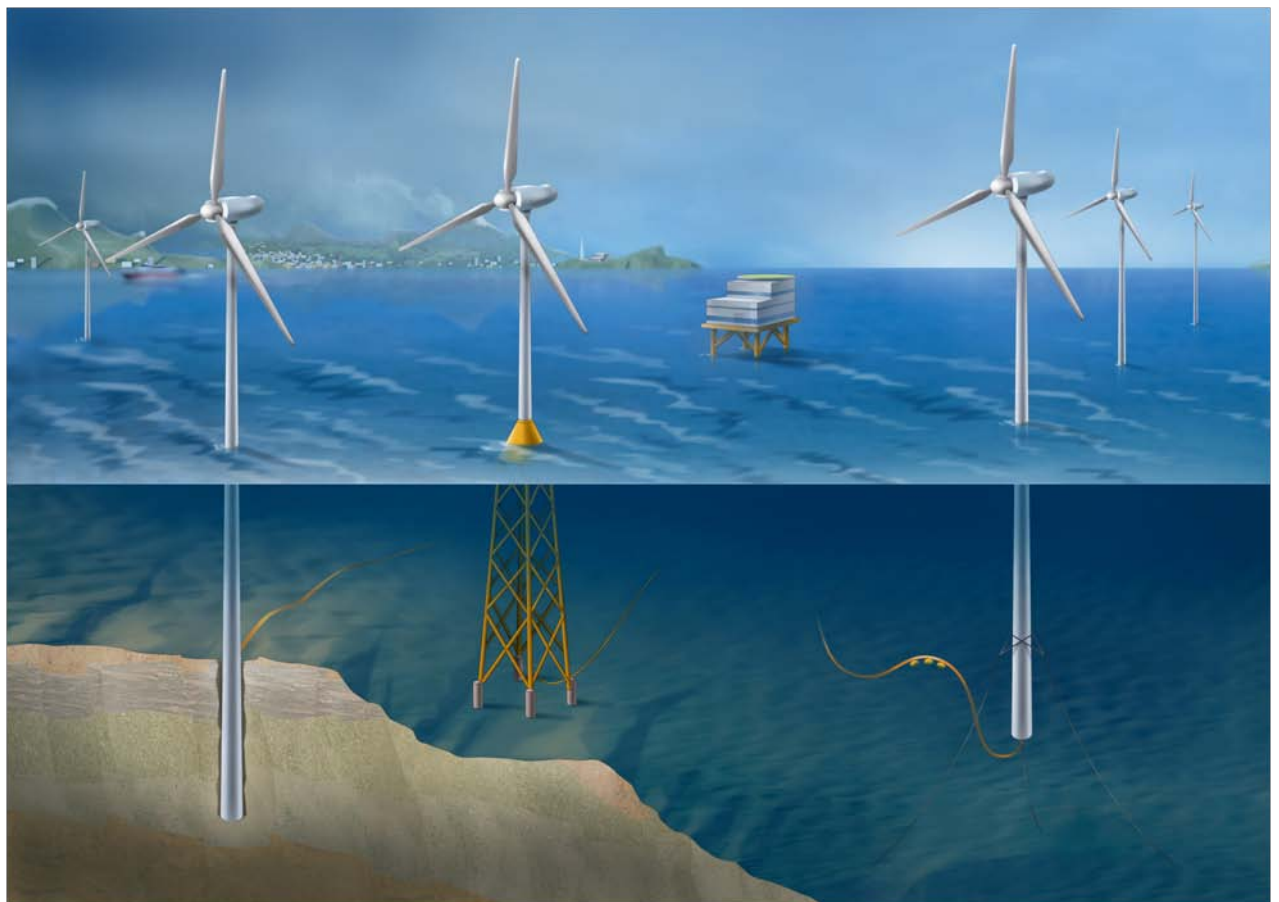
Figure 1 Illustration of offshore wind turbines with different sub-structures, from left: mono-pile, jacket and floating spar.
