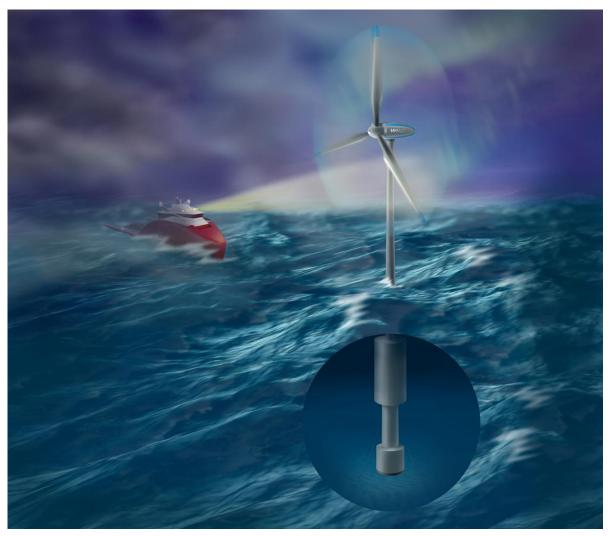
**Figure 1** Illustration of an offshore wind turbine on a floating spar sub-structure together with a vessel.
