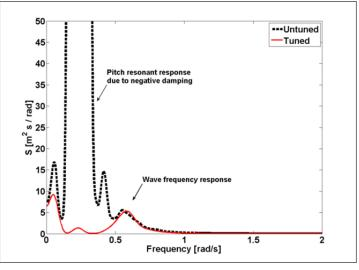
Figure 11 Spectrum of nacelle surge motion of a tension leg spar (TLS) with a downwind wind turbine under simultaneous wind and wave loading, and operating at an above rated wind speed. By tuning the controller, the pitch resonant motion was reduced, and the power production was significantly improved. (From Dr. Madjid Karimirad's thesis.)
