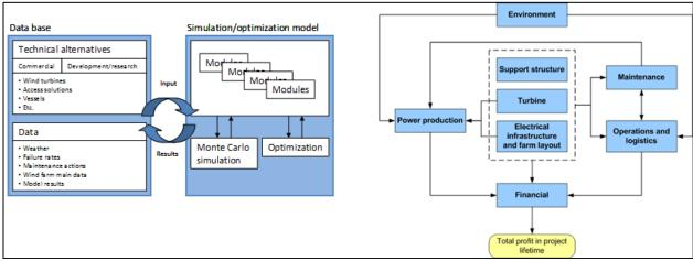
**Figure 13** Holistic/integrated model concept for Life Cycle Profit analysis of an offshore wind farm, including all phases from design to decommissioning (Task 5.1).
