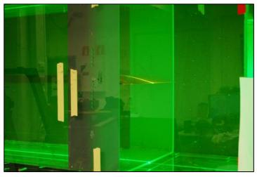
**Figure 15** An airfoil model mounted wall-to-wall in the circulating water tank for PIVexperiments. The experiment was carried out to investigate the effect of scaling in model tests. The measurement plane is vertically orientated in mid-span position.
