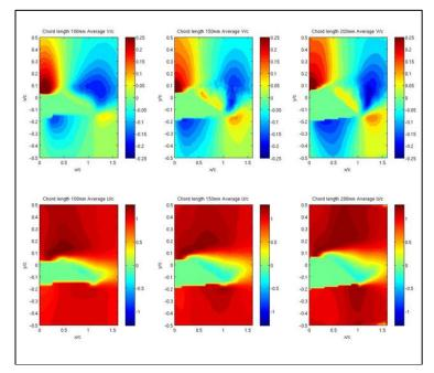
**Figure 16** Results from the PIV-experiments in the circulating water tank. The plots show the horizontal and vertical velocity component near the trailing edge of an airfoil tested at three different model scales.
