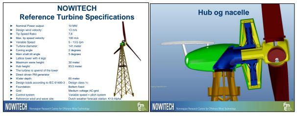
**Figure 7** NOWITECH reference turbine. Summary of specifications (left) and extract from hub and nacelle construction (right).
