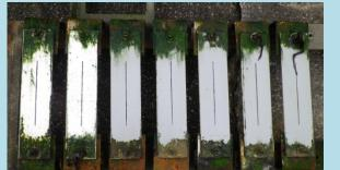
Coating systems combining thermal sprayed zinc and a paint applied in 1-coat instead of a conventional 3coat paint system show promising corrosion performance in a field test at Helgoland.
