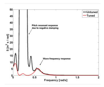
These results show that negative damping adversely affects the performance and structural integrity of a floating wind turbine and should be avoided.
