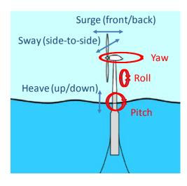
The motions of a floating wind turbine are defined by the six degrees of freedom:
