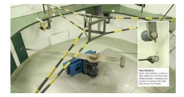
SAAB Rain erosion test facility
