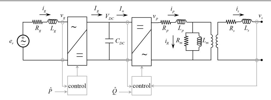
Inner-loop generator-side converter control
