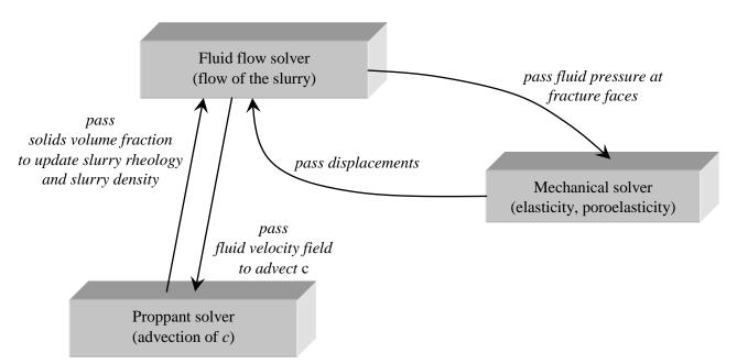
*Figure 3.1* Coupling of different building blocks of a hydraulic fracture simulator. Thermal solver is omitted to avoid cluttering in the Figure.
