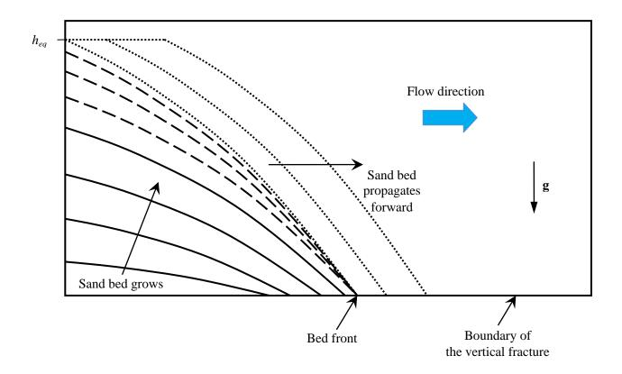
*Figure 1.1* Growth and propagation of sand bed during proppant injection into a vertical hydraulic fracture.
