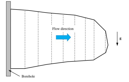
*Figure 2.1 Fracture discretization employed in simplified proppant transport and settling models.*
