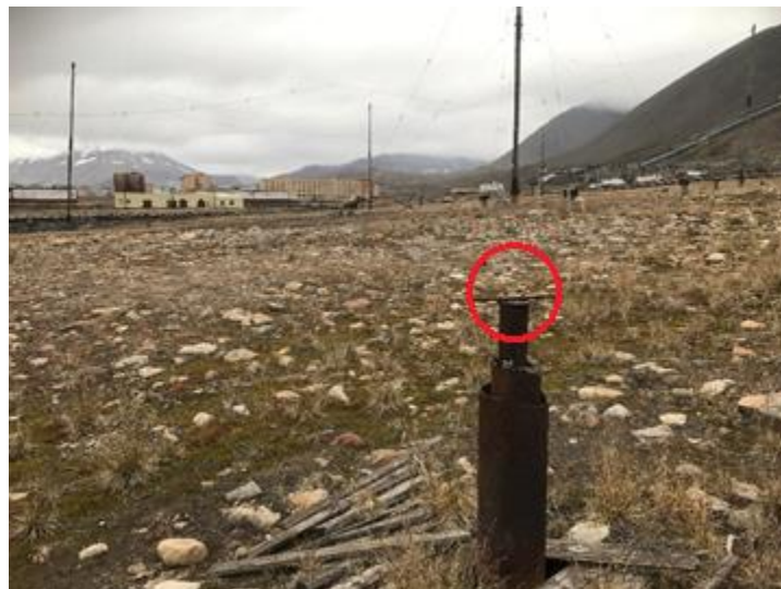
Figure 31. Reference point N3 (PRP3), circle points the bolt, on which the bar staff was placed for surveying.
