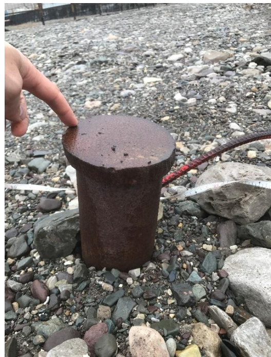
Figure 30. Reference point N1 (PRP1), finger pointing at the upper point of the platform, where the rod (barcode staff) was placed for performing the measurements.
