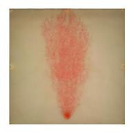
2D-cell experiment illustrating the buoyant migration of  $CO_2$  in an aquifer (Polak et.al., 2010). (Photo: SINTEF)
