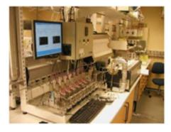
Gas permeation unit for testing of high temperature dense hydrogen selective membranes. (Photo: SINTEF)
