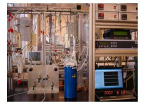
Ebulliometer for characterization of amines. (Photo: SINTEF)
