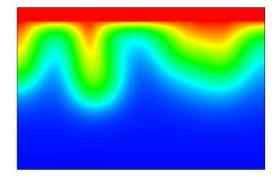
Computer model of convection patterns in water under a CO<sub>2</sub> gas cap (Wessel-Berg, 2009). (Illustration: SINTEF)
